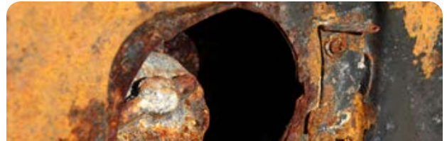
UNDER-DEPOSIT CORROSION IS HALTED ONCE BIOFILM IS REMOVED.
